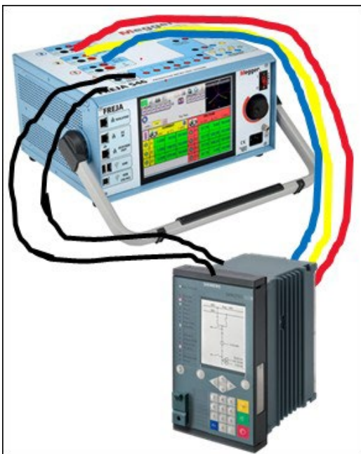
Figure 2: Simplified diagram of a relay test set physically connected to a protection device for performing protection tests.
