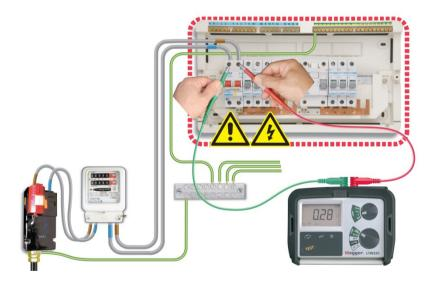
Loop impedance, either earth loop or line-neutral, will have a greater influence on the PFC/PSCC value the smaller they get, causing issues when taking measurements below the stated range of an instrument. Any PFC measurement should be taken using the high current option – no-trip test ranges should only be
