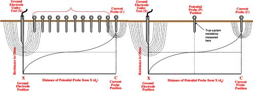
When testing a single earth electrode the C spike can usually be placed 15 m away from the electrode under test, with the P spike placed 9m away. With a small grid of two electrodes, C can be placed about 100 m from the electrodes under test; P spike about 62 m away. Larger earth systems consisting of several rods or plates in parallel required the distance for C to be increased to possibly 200 m and P to some 125 m.
