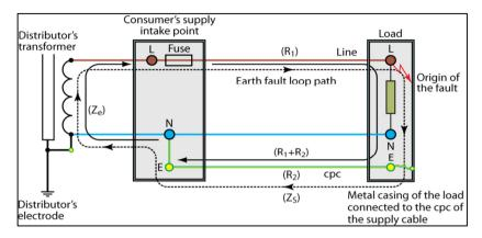
Earth fault loop return path – TNC-S installation
