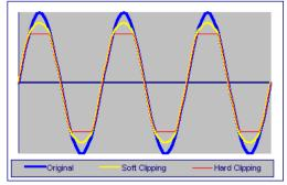
Harmonic disturbance – This has now earned the right of a section within the 17<sup>th</sup> Edition and the problems severe harmonics can cause are being formally documented to a far greater extent. The detrimental effect on a loop test signal can be significant, but repeat testing, again, can often overcome this.
