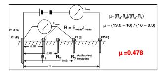
The resulting value of u (which in this example = 0.478) is then looked up in the table shown below. In this example the correct earth system resistance would be measured with the P spike at 0.632, or 63.2% of the C spike distance from the electrode under test.
