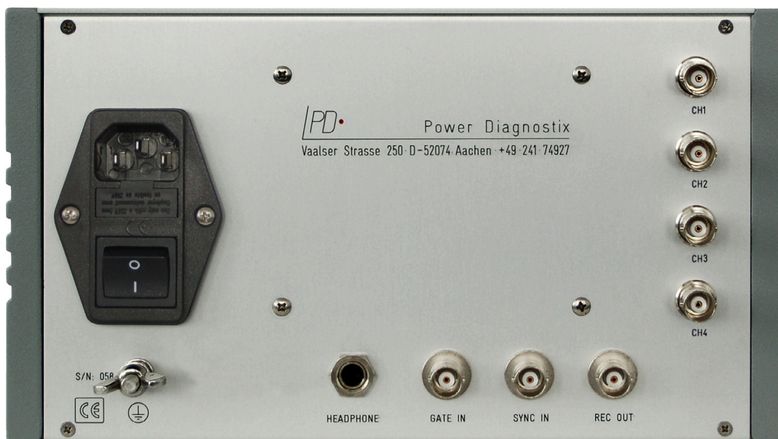
Figure 3.2: Rear panel of the AICompact 1/2 19-inch model
