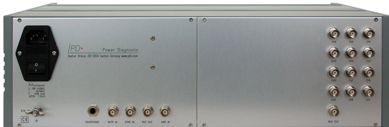
Figure 3.4: Rear panel of an 19-inch AICompact with 12-channel multiplexer
