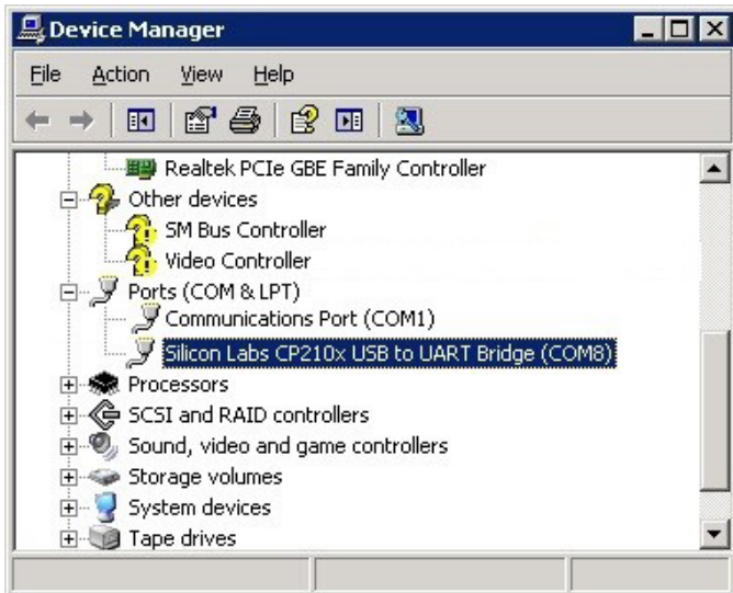
Figure 8.3: Windows Device Manager items after a successful driver installation
