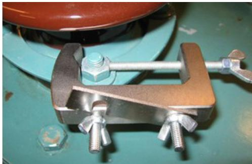
The sharp, adjustable M4 pin screw penetrates any paint or oxide, making it easy to get a good, solid ground connection on almost any surface.
