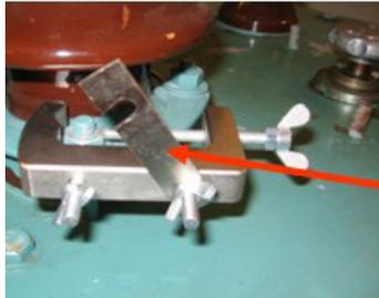
To attach and tighten the braid: open up the braid plate by loosening the wing nuts.
