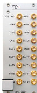
Figure 5: Disturbance combiner unit (DCU4)
