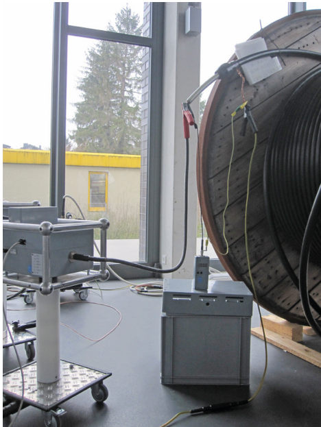
Figure 57: CAL1B connected to MV cable (lab)
