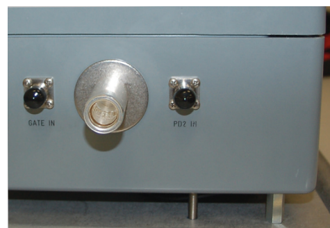
Figure 93: Additional input for noise cancellation 'PD2 IN'
