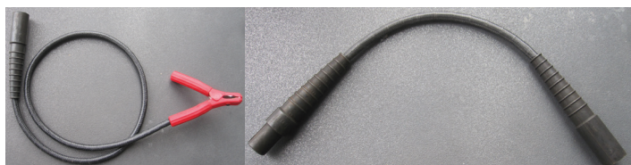
Figure 3: High voltage cables
