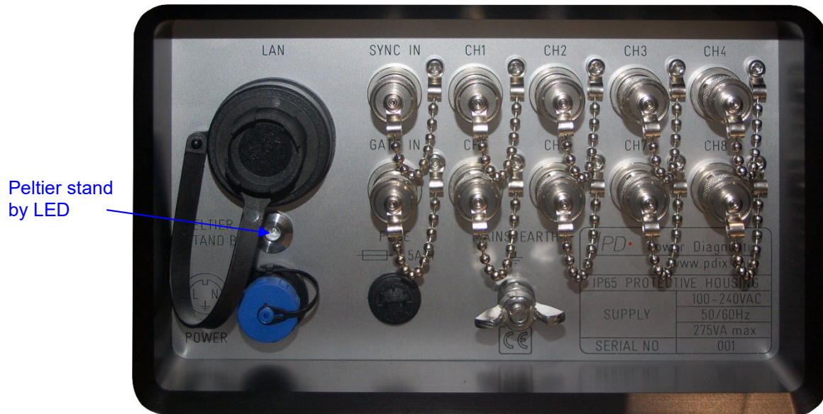
Fig. 3: Connection panel with protective caps attached to connectors
