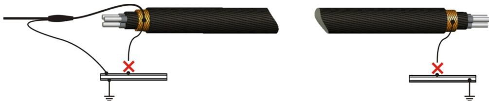
The insulation of any high or medium voltage shielded power cable is protected from water ingress by a jacket made from XLPE or PVC. The Sheath test
