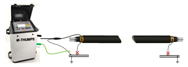
The insulation of any high or medium voltage shielded power cable is protected from water ingress and mechanical damage by a jacket made from XLPE, PVC etc. The Sheath test checks *if* the integrity of the jacket has been compromised, typically during installation.
