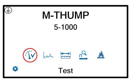
The main screen image shows can show up to 5 icons for different operation modes. More modes can be selected by the user in the expert mode under "UNIT CONFIGURATION", in this case the displayed icons represent *types of operation (in this example PRELOCATION)* and by clicking on them display the individual modes
