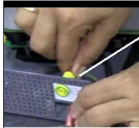
**Disconnect the ground and power on off switch connectors**
