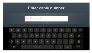
Entering the cable number as accurately as possible makes it easier to assign the cable later when reporting and archiving the measurement data record in the reporting software. If this kind of further processing is not planned, the cable number does not have to be entered. Regardless of whether or not a cable number has been entered, confirmation via is required.
