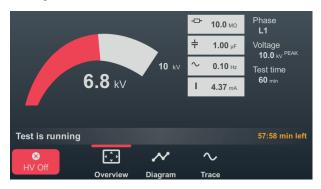
In addition to the current test voltage and the remaining test duration, this also displays the following measured values depending on the operating mode:
