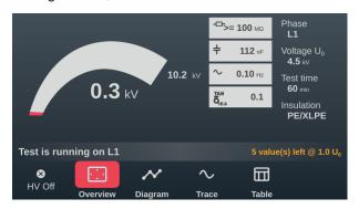
In addition to the current test voltage and the remaining test duration (or the remaining measured values in the step test), this also displays the following measured values:
