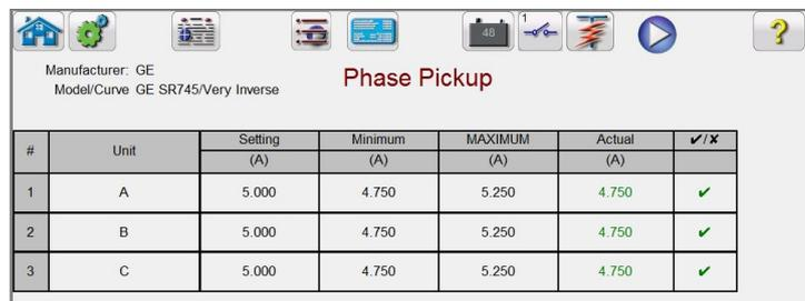
The screenshot shows the 'Phase Pickup' measurement screen. At the top, it displays 'Manufacturer: GE' and 'Model/Curve: GE SR745/Very Inverse'. Below this is a table with the following data:
