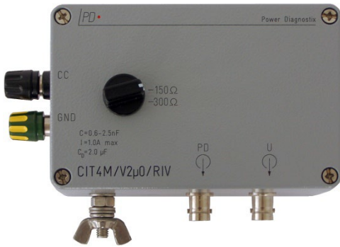
Fig. V.46: Quadrupole suiting both NEMA 107 and CISPR 18–2 impedance requirements
