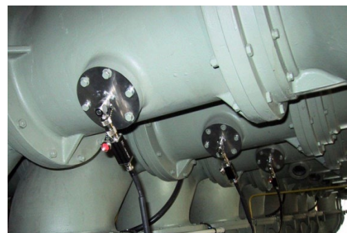
Fig. V.21: Windows sensor with FCU2
