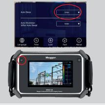
Select a time setting from the **Auto shutdown** drop down menu. The device will automatically shutdown if there is no user input for the specified time.
