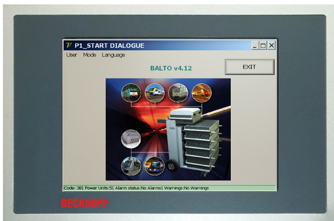
Abb. 19: Bedienfeld: Touchscreen-Display – HMI
