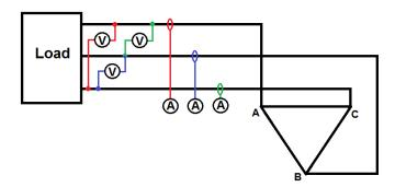
The 3 phase voltages and 3 line currents can be measured and then the power can be calculated mathmatically by using the  $\sqrt{3}$ . This will calculate the proper power values provided the delta is balanced. The more unbalanced the delta is, the more error is introduced into this type of measurement. A 2 wattmeter method will provide accurate values regardless of how well balanced the delta is.
