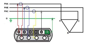
Note the connect Phase C voltage to the N input of the analyzer. This is because it is used as the reference.
