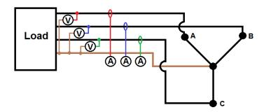
When measuring a delta, all the voltages are referenced to other lines; there is no neutral. This means the measured voltage in a delta are phase voltages. The measured currents are still line currents. Since the voltages are phase voltages but the currents are line currents, the measurement itself introduces a 30-degree phase shift.
