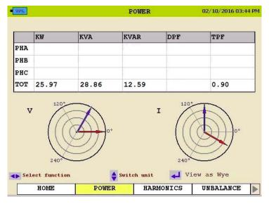
This screen displays the total power going to the load. It also displays the phase voltage versus line current phase angles.
