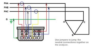
Note the channel 3 voltage input is connected across phase a-b.
