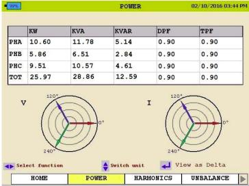
This will get the power going through each phase and the phase angles between the phase voltages and phase currents.
