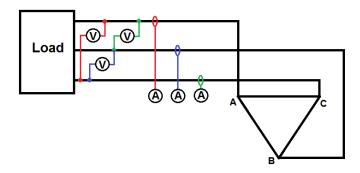
The 3 phase voltages and 3 line currents can be measured and then the power can be calculated mathmatically by using the  $\sqrt{3}$ . This will calculate the proper power values provided the delta is balanced. The more unbalanced the delta, the more error is introduced into this type of measurement. A 2 wattmeter method will provide accurate values regardless of how well balanced the delta is.
