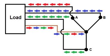
In a delta, the power flow return is on one of the phases.
