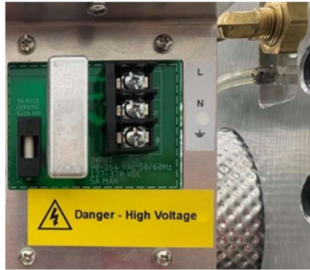
Figure 1: Input Power Board
