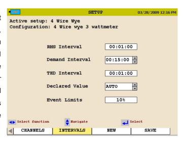
In this screen, you can also change the declared voltage value. When set to AUTO, the MPQ will automatically measure the declared voltage. If you want to set it to a specific value, use the arrow keys to navigate to the declared value field and make the proper selection.
