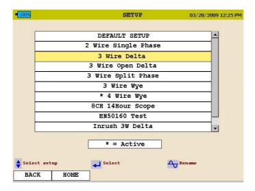
In the "NEW" screen, you can select and activate different setup files. Choose from a selection of default setups with different power configurations, select an inrush test, select a recording scope mode to record nothing but waveforms for months on end or activate a custom setup file you create in the PC software.
