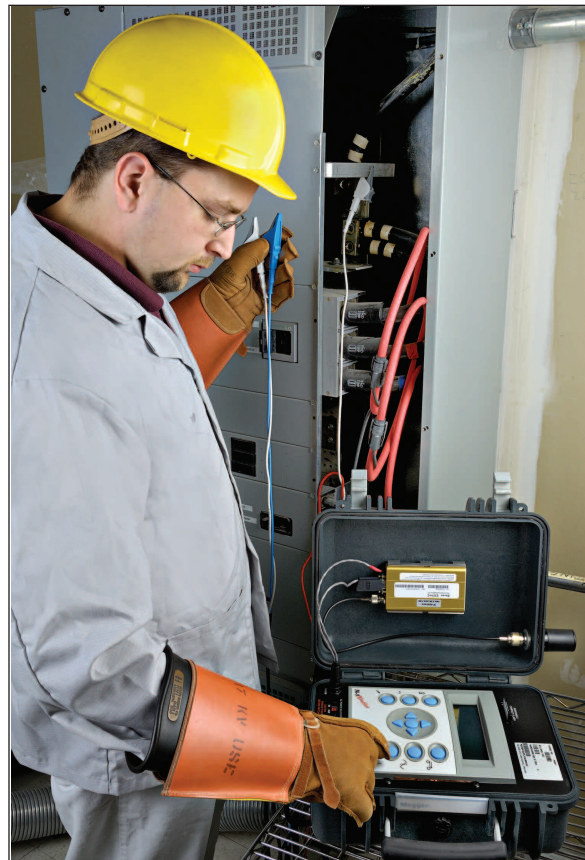
The PA9Wireless is quick to install and easy to use. Everything needed to remotely monitor power and power quality is included in one package.
