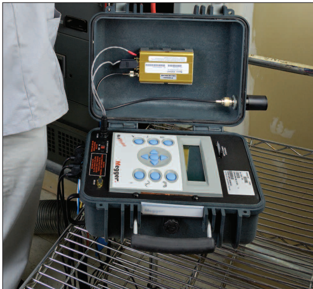
The PA9 Wireless incorporates both a Raven Cellular Modem and antenna built into the lid, providing easy, effective remote communications.
