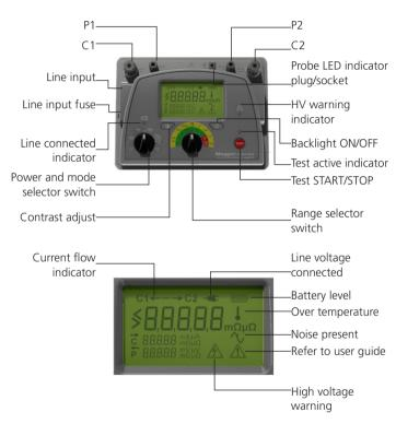
After starting a test the user will see confirmation of successful continuity testing on the LCD. If the dashes are not shown connecting 1 & 2 C and/or P leads connection has not been detected.
