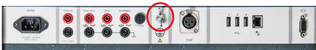
Figure 1.2-1 Protective conductor terminal
