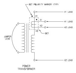
Figure 5-7. Setup for Testing BCT Mounted on Single-Phase Two-Winding Transformer
