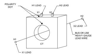
Figure 5-5. Setup for Testing Unmounted Current Transformer
