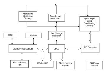
Figure 4-1. Single-Phase TTR Test Set Block Diagram
