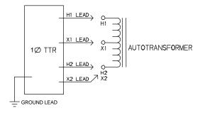
Figure 5-2. Setup for Testing Single-Phase Autotransformer
