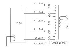
Figure 5-6. Setup for Testing Taps on Multiple Tap CT
