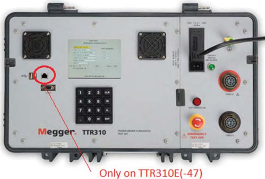
Figure 4-2. Three-Phase TTR310 Control Panel
