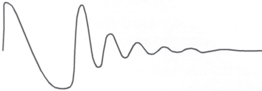
Fig 2: Example of a “ringing” wave pattern resulting from Surge Testing.
