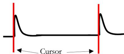
With Pulse Echo, the output pulse travels twice the distance of the cable. i.e. from the output of the TDR to the change of impedance and the returning reflection back to the TDR., so the length to the impedance change is shown as:
