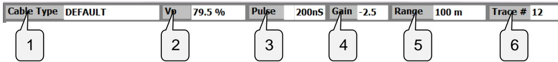
1. **Cable Type:** Selected from cable library, or custom cable put in by operator
