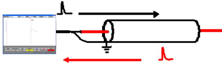
From these low-voltage pulses, a small amount of energy is reflected back to the TDR from a change of impedance and is displayed on the MTDR screen, as either a positive going or negative going pulse, depending on the impedance characteristic (negative pulse for low impedance to shield faults and positive pulse for high resistance faults).
