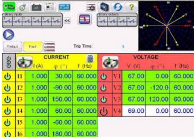
Figure 1 Advanced Manual Test Screen for a 5 Channel, 4 Voltages / 6 Currents Unit
