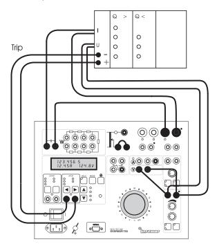
Q: Reactive power  $\alpha$  = 90° (phase-shifting capacitor in current circuit)
