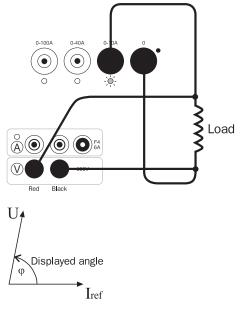
**B**] Current generated by external source (ammeter panel input used).
