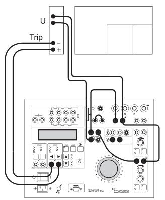
Sometimes it is necessary to change between two voltage levels and measure the time that elapses until operation. This can be done using the SVERKER make/ break contact.
