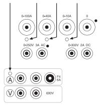
Use the button marked A to transfer the ammeter test point to the selected input.
