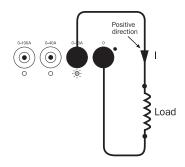
**B**] Current generated by external source (ammeter panel input used).
