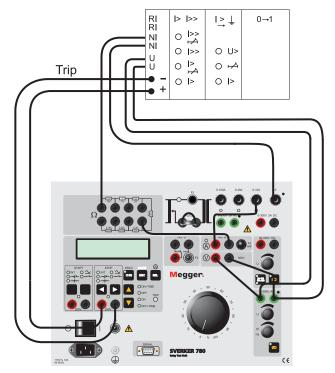
Connect for testing as shown in the above diagram.
