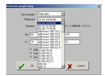
**2**] In the Reference Graph setup you can select "Relay type" and use one of the ready-made relay curves for a specific relay instead of a characteristic.
