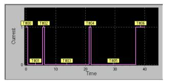
This is a test of an overcurrent relay with autoreclose.
