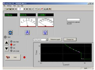
This is the SVERKER Win window from which you control most of the test. The "*Comments for selected trip point*" field is used if you want to write a comment to the actual test shot, e.g. Pick-up test, this will then be printed in the report on the same line as the test shot.
