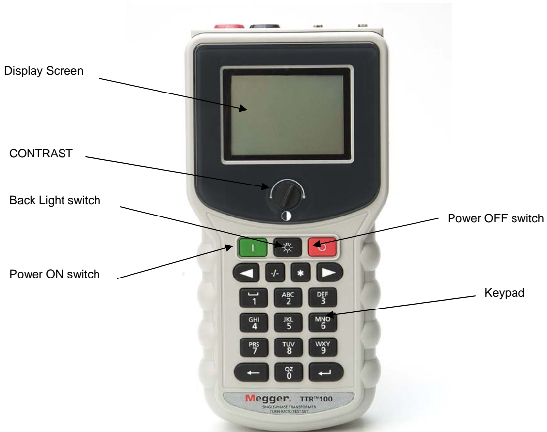
Figure 4-1 Single-Phase TTR Display & Control Panel
