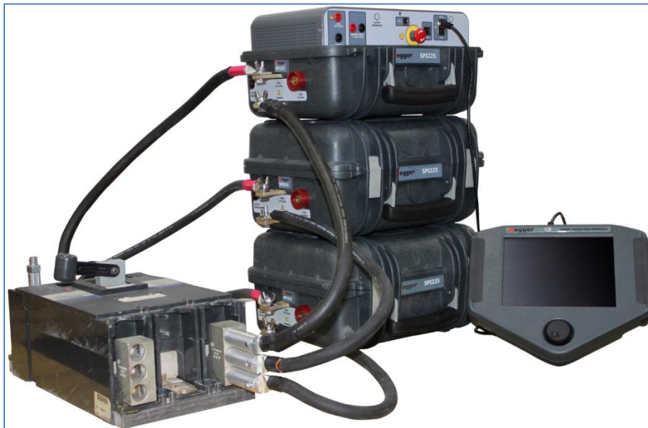
Figure 24 - Three SPI Units in Parallel
