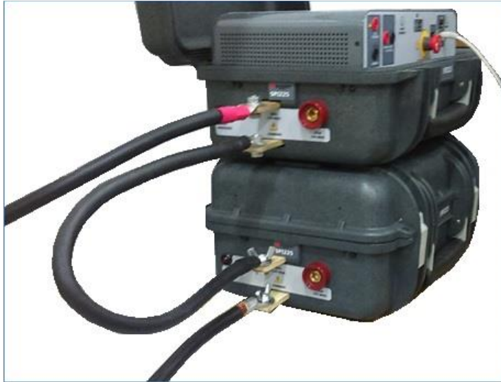
Figure 25 - Series Connection of Two SPI Units
