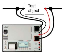
Fig. 5.1 On MJÖLNER 600 the current outputs have reverse position.
