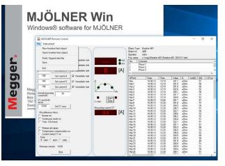
The MJÖLNER Win program makes it easy to manage/ save all test results in a simple way. All information, meta-data of the test object e.g. a circuit breaker and the test results are stored together and they can easily be transferred to Microsoft® Excel for further analysis. In MJÖLNER Win you can also save test files and print out test reports.
