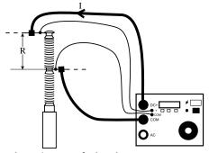
Measuring the resistance of a breaker
