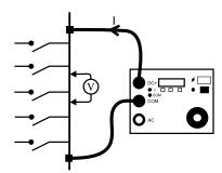
Measuring resistance at busbar joints
