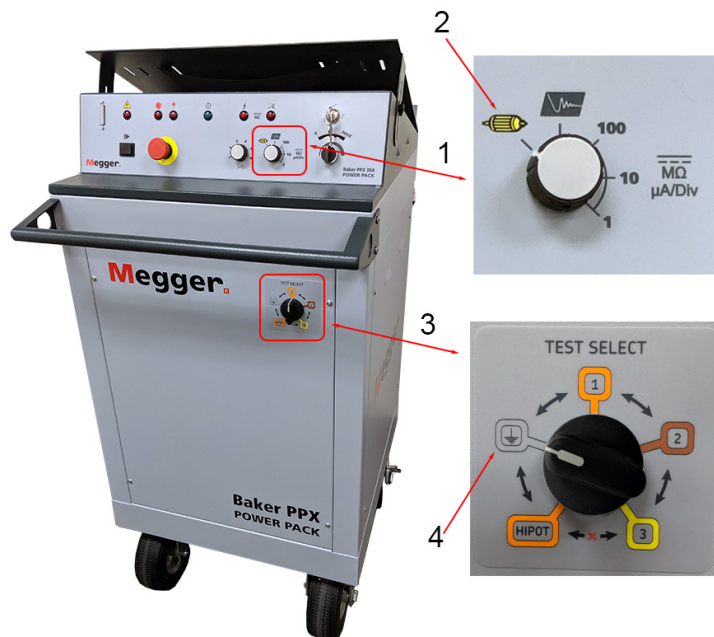
Fig 39: Baker PPX30A armature test settings.
