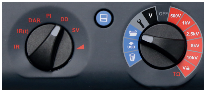
Modern mode and function switches on insulation tester
