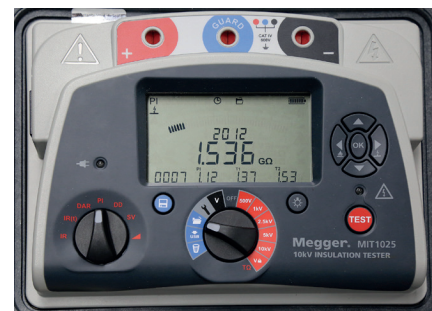
Results of Polarization Index test on MIT1025 10kV insulation tester
