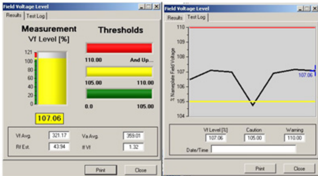
Fig 113: Field Voltage Level.
