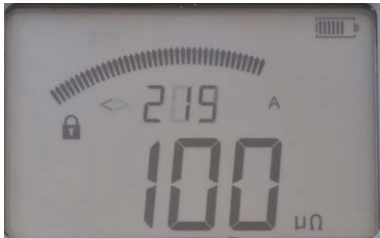
Max current during test was 219 A.
