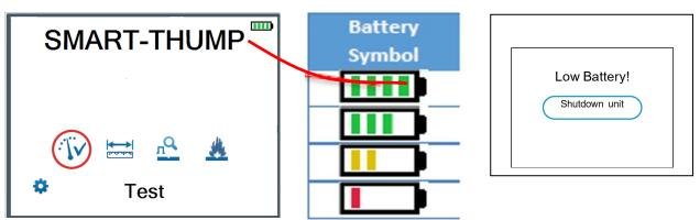
NOTE: To protect the battery from a deep discharge, the unit turns off automatically completely or provides an error message if the battery is discharged too low for safe operation, see above.
