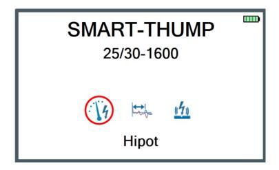
The main screen image shows a typical set up with the 3 basic elements of fault locating, HIPOT, ARM PRELOCATION and PINPOINTING (other elements or modes of operation can be set up; an additional icon for each selected mode will show on the main screen).
