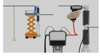
Measurement on circuit breaker with one side grounded. Here is a combination of one clamp and one probe used
