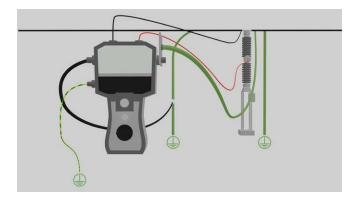
Traditional measurement from ground. Injection is done through existing grounding cable (earthing). use any of the optional cable kits, GA- 00380/82/84 with 5,10, or 15 m cables.
