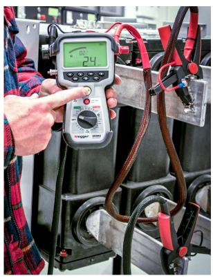
Hold probes / attach Kelvin clamps to CB and press trig / TEST button. A signal indicates whether test was pass or fail and result is logged in unit for later dump to PC.
