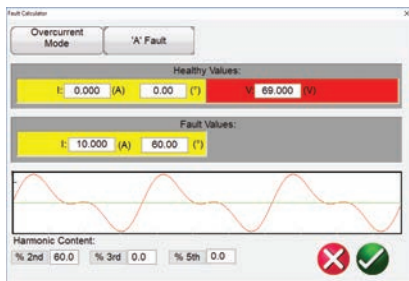
Figure 3 Fault Calculator with 2nd Harmonic
