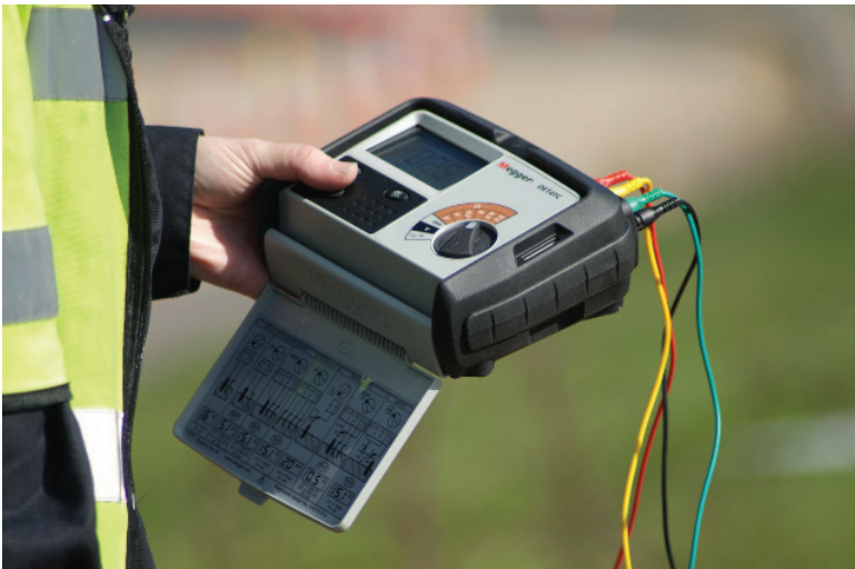
Using a Megger DET4 series to test building earth (ground)
