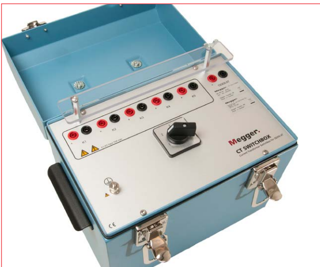
Current transformer switchbox BH-90130 The Current Transformer (CT) Switchbox for ODEN AT is a tool that is used to facilitate CT testing. The secondary windings on the CT are connected to the CT Switchbox inputs and output is connected to ODEN AT Ammeter 2 terminals. The switch is used to select which secondary winding on the CT that should be measured. The windings that aren't measured are short-circuited. Up to five secondary windings can be handle.
