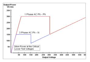
PowerV<sup>™</sup> technology guarantees a flat curve from 30 to 150 V, eliminating range switching
