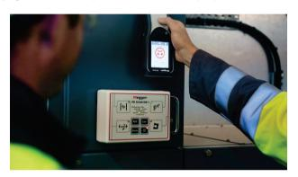
The box starts operating directly after being switched on, and generates partial discharge-like pulses. The level and frequency of the pulses, as well as the type of decoupling, are based on the current settings, which can be adjusted as following using the buttons on the front panel:
