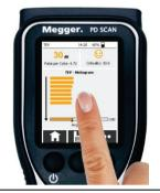
The measurement is paused and the current measurement results are frozen. If headphones are connected to the device, then the acoustic, audible signal is also muted. Instead of the button, the button used to continue the measurement now appears at the bottom edge of the screen. Briefly tapping the display again also allows the measurement to be continued.
