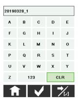
Briefly pressing the button allows the user to scroll through the list of fields on the touch screen. Pressing the Pressing and holding the button deletes all characters. You can switch to the numeric keypad by pressing 123. In addition to number keys, the keypad also has six freely assignable keys for frequently used text modules.
