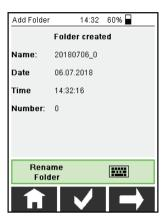
A new folder is created, the name of which is comprised of the current data and a running index.
