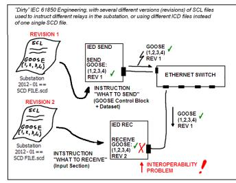
A typical example of this interoperability problem is a difference in the configuration revision of the GOOSE message. In the SCL file there is Configuration Revision 3, and the published GOOSE has configuration revision 2.
