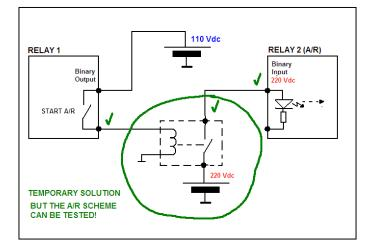
By doing this conversion, which simply requires one auxiliary relay and one power supply at 220 Vdc, the protection scheme between the two relays can be tested and the commissioning of the substation does not suffer unnecessary delays.
