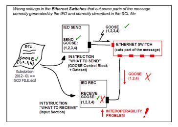
This interoperability problem can occur in multi-vendor but also in single-vendor applications. A typical example is illustrated in the VLAN tag of the GOOSE message, that is removed (or altered) by the switch (or switches), depending on the VLAN settings of the switch itself.
