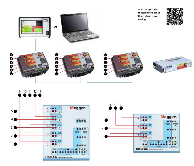
The SMRT test sets shown are connected via standard RJ45 Ethernet cables and controlled from a single STVI interface or PC. This example presents a 32-channel testing environment.
