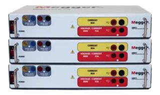
You can connect three SMRT1 units for three-phase testing (3 x 300 V at 150 VA plus 3 x 60 A at 300 VA) and they still weigh less than 30 lbs!
