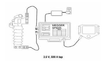
have a pre-fault setting is often required when testing small self-powered reclosers for proper operation. The SPI225 can operate on 120 V or 240 V and is the most compact test set for testing self-powered reclosers on the market.
