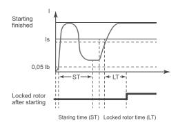
Case of locked rotor after starting.
