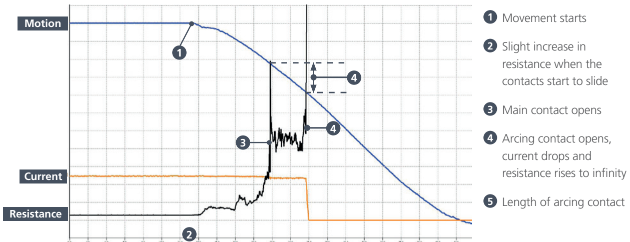
DRM is a reliable method to estimate the length/wear of arcing contact
