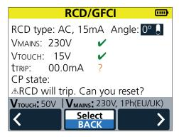
Should a red FAIL result occur the charger the trip level is of concern and will most likely result in nuisance tripping of the RCD or GFCI is use. A qualified electrician should be consulted.
