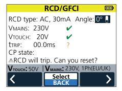
Should a red FAIL result occur the charger should be taken out of use until a new RCD / GFCI can be fitted.
