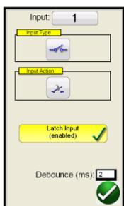
The default settings are Binary Input 1, dry contacts as indicated by the Input Type, and Input Action defaults to show the Closing of the Normally Open contacts. To change the Input Type from dry contacts to Voltage, press the Input Type Transducer button, and it changes to voltage. To change to the opening of Normally Closed contacts press the
