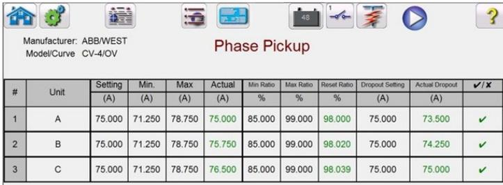
Figure 136. Example Phase Pickup and Dropout Test Screen
