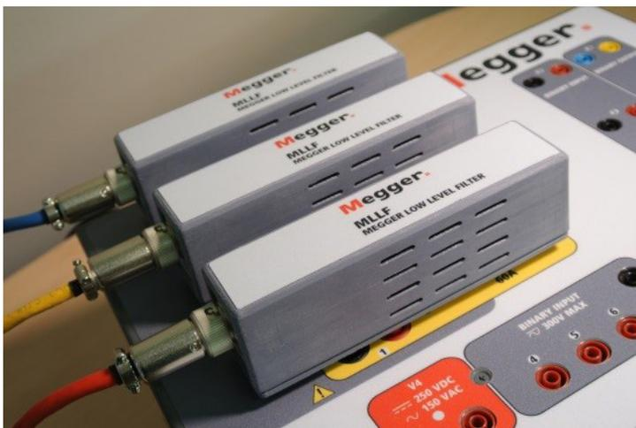
Figure 15. MLLF Megger Low Level Filter modules
