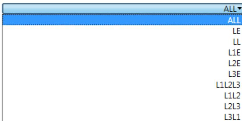
Figure 189. Defining Fault Type for Impedance Characteristic
