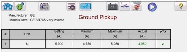
Figure 121. Example Ground Pickup Test
