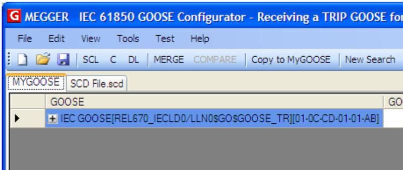
Figure 283. Imported GOOSE in MyGOOSE for Mapping
