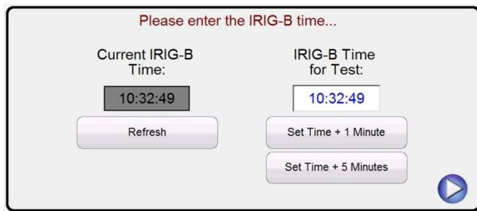
Figure 246. Setting IRIG-B Trigger Time
