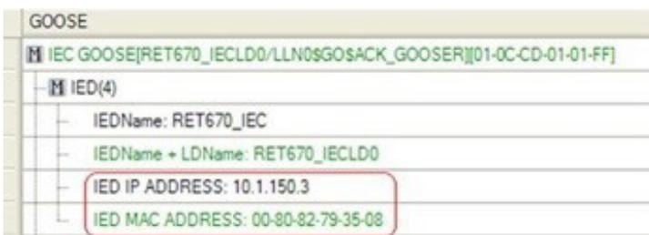
Figure 272. IED IP Address in the SCL File
