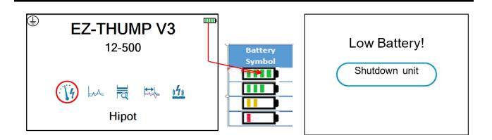
*NOTE:* To protect the battery from a deep discharge, the unit turns off automatically completely or provides an error message if the battery is discharged too low for safe operation, see above.
